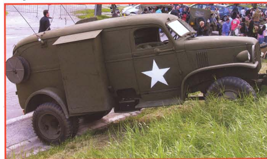
Above: Campanini's 1-1/2 ton Chevrolet 4x4 K51 radio truck parked near the DUKW exhibition.
